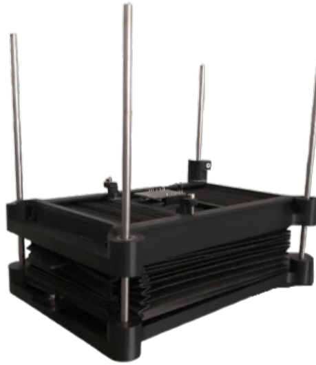
Figure 2. Custom 3D-printed data acquisition rig with a camera mount repositionable in all three axes
