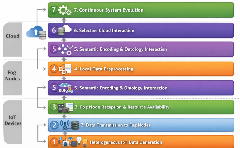
Figure 1. Overall system model of the proposed fog-based adaptive semantic interoperability mechanism
