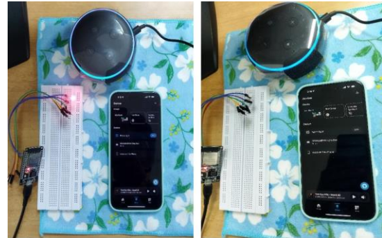
Figure 9. Controlling Esp32 C3 using a Amazon Alexa voice assistant
