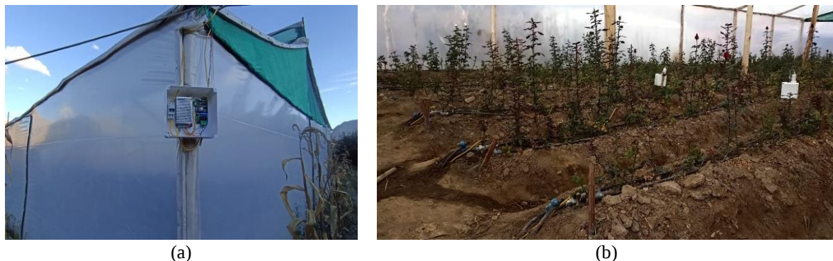
Figure 7. Implementation inside and outside the greenhouse; (a) the CN and (b) the SNs with solenoid valves
