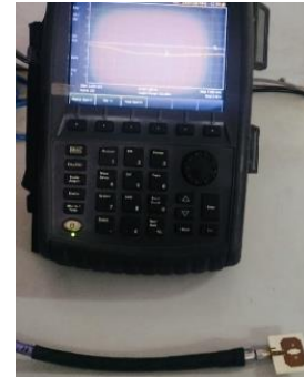
Figure 12. Proposed antenna connected with VNA to measure the S11 parameter
