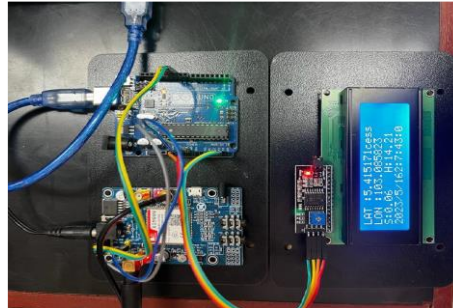
Figure 8. Prototype of WDC tracking device
