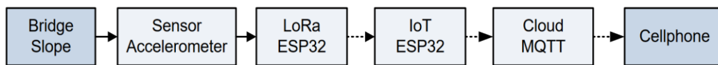
Figure 1. System model for early detection of bridge slope using LoRa and IoT
