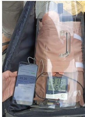
Figure 14. Temperature and humidity values of DHT21 sensor and digital thermometer in neonate incubator room
