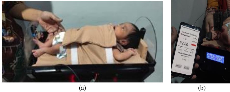
Figure 15. Testing the DS18B20 sensor in the neonate incubator room (a) a one-week-old newborn baby and (b) the temperature value on the heating application and the LCD of the portable neonate incubator
