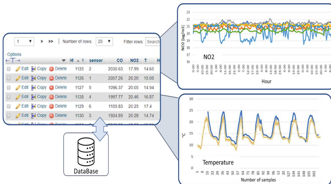
Figure 10. Data storage and visualization with the web application
