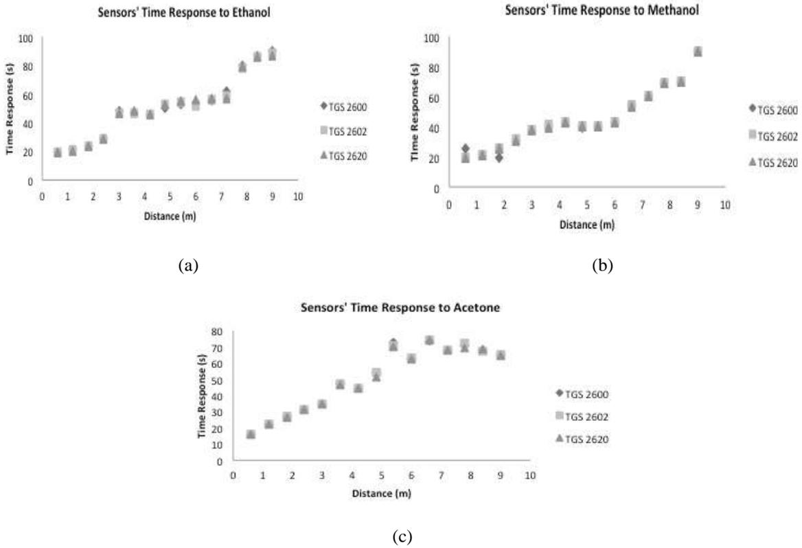
Figure 4. Sensor's time responses to some sources(a) to the ethanol, (b) to the methanol, and (c) to the acetone
