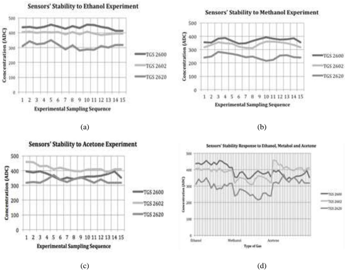
Figure 7. Sensor's stability for 3 different sources (a) ethanol, (b) methanol, (c) acetone
