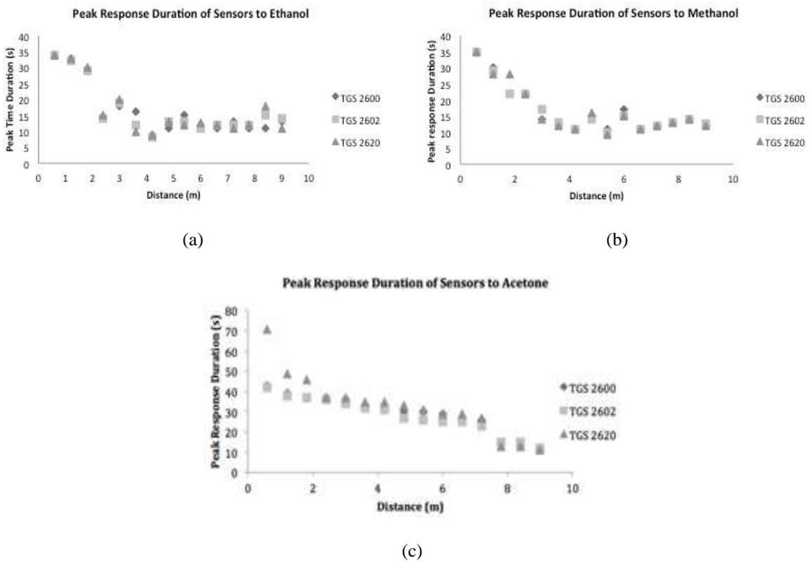
Figure 5. Sensor's peak duration responses for 3 different sources (a) ethanol, (b) methanol, (c) acetone
