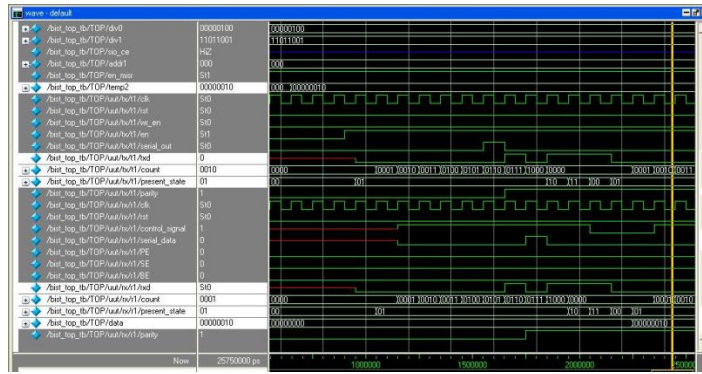
Figure 9. Simulation Result of UART Transmitter and Receiver
