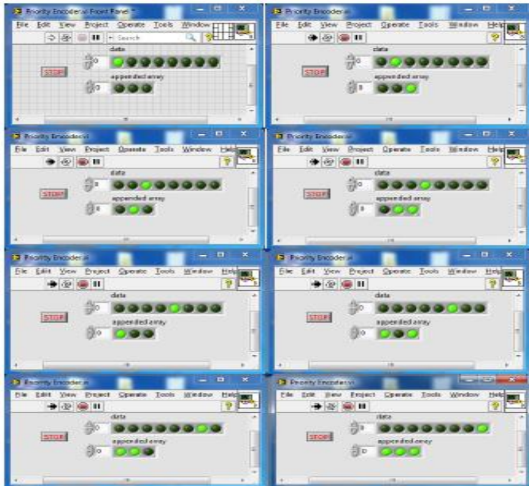
Figure 11. Priority Encoder LabVIEW output waveforms
