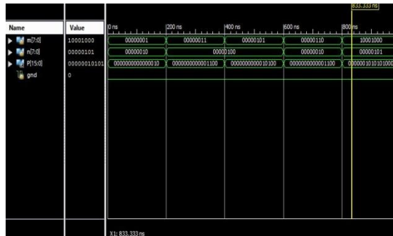
Figure 6.1. In the above figure m[7:0] and n[7:0] are the inputs and P[15:0] is the product. The result is shown by 4-2 compressor
