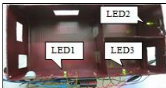
Figure 9. LEDs light up when value of light intensity less than 40
