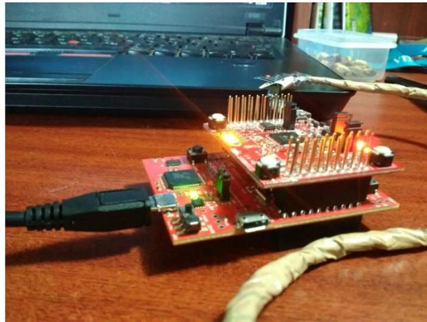
Figure 7. Wi-Fi module with Launch pad
