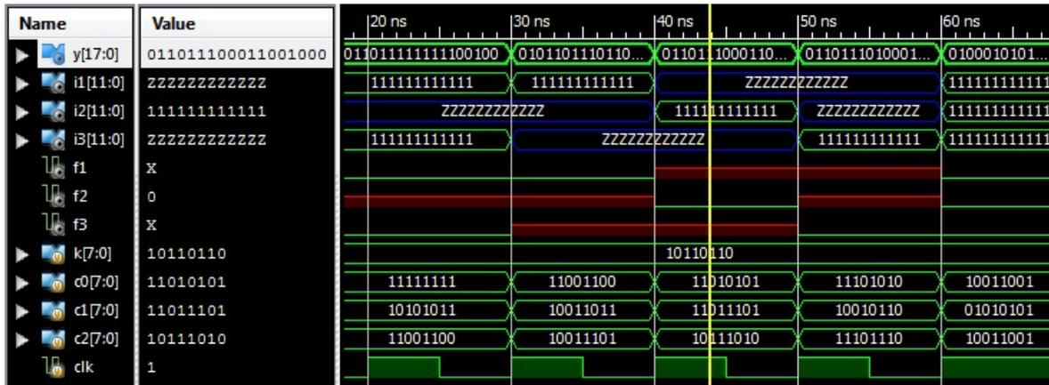
Figure 5. Simulation waveforms for FIR filter before fault injection
