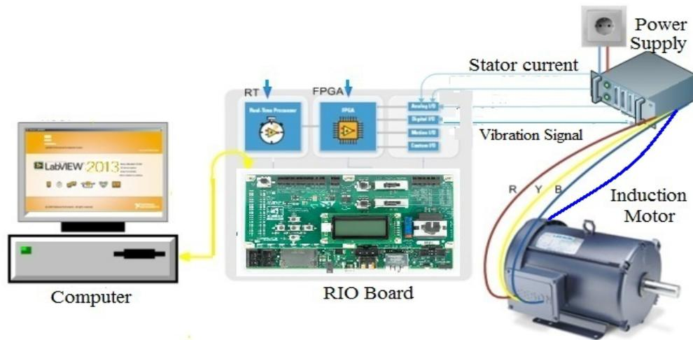
Figure 6. Test environment used for the development reconfigurable system
