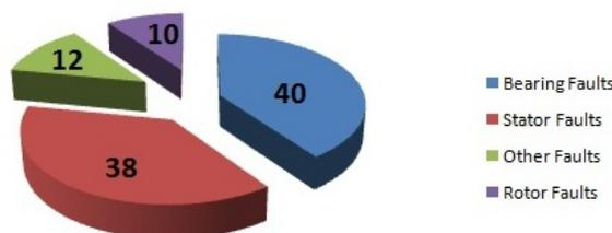
Figure 1. Fault Percentages in Induction Motor
