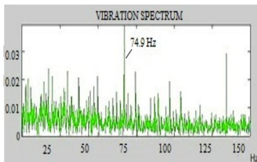
Figure 8. Vibration spectrum for outer race fault
