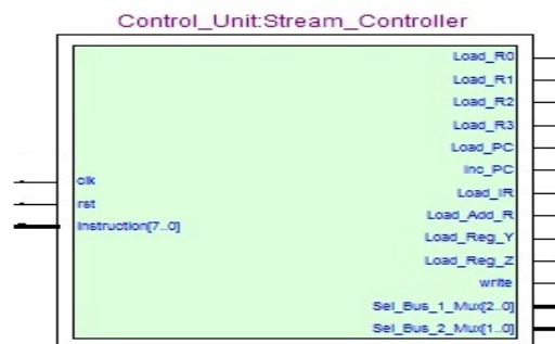
Figure 10. Generated Block Diagram of the Stream Controller
