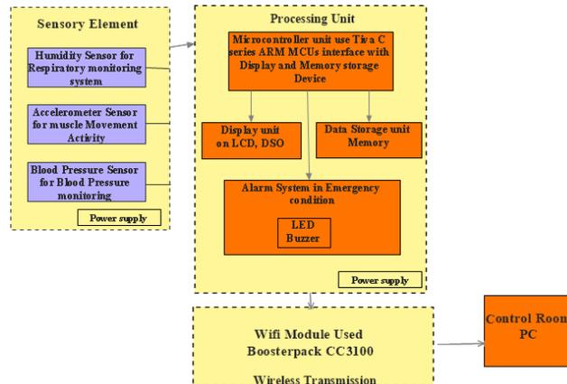
Figure 4. Block diagram
