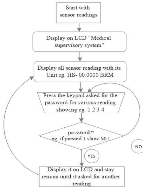
Figure 3. Algorithmic Flow chart for displaying the output
