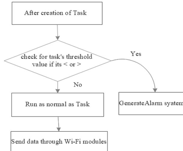
Figure 2. Tasks Generating Interrupts for alarm system
