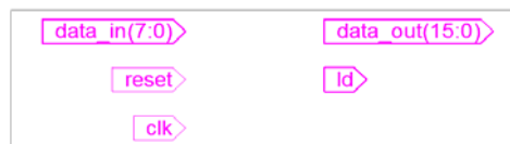
Figure 1. In-out schematic of low pass & high pass FIR filter modules
