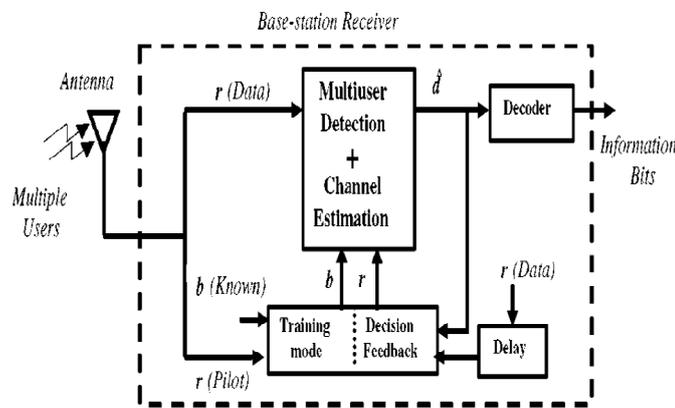
Figure 1. Simplified view of the base station receiver. This figure shows the several user channel assessment and detection blocks in the receiver. A training sequence (pilot) is used for channel assessment and decision feedback is used to update the assessments in the absence of a pilot.
