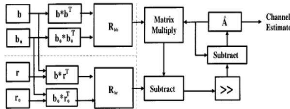
Figure 8. Time-constrained VLSI architecture block diagram. The dotted lines show the parts corresponding to. All operations within a block are being computed by exploiting the maximum parallelism available in that block. The parallel matrix multiplication.
