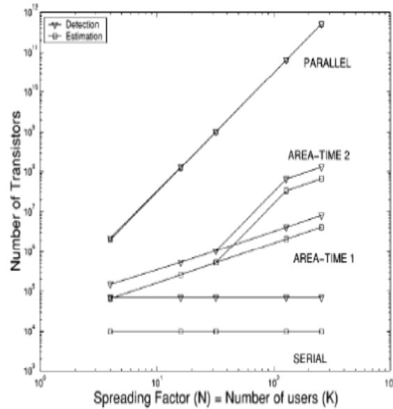
Figure 7. Area requirements for different VLSI architecture tradeoffs with varying spreading gains. Ashows the number of transistors required for a serial, a parallel and two data rate tradeoff architectures with 16-bit precision.
