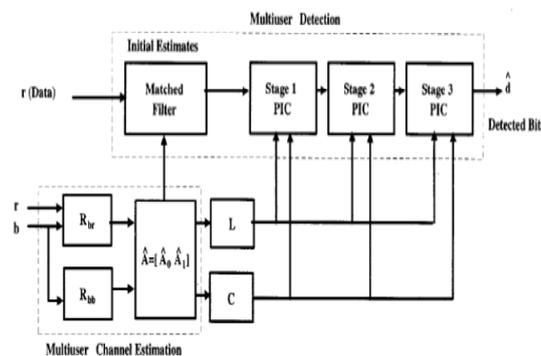
Figure 5. Task decomposition of joint multiuser channel assessment
