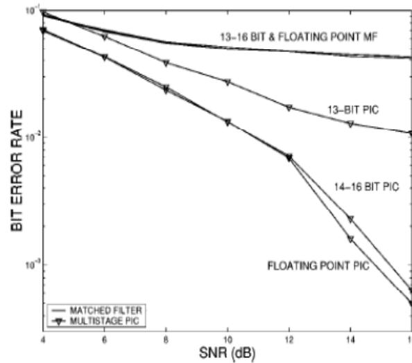
Figure 3. Fixed point error rate performance for  $N = 16$ ,  $K = 8$ . The figure shows the effects of quantization on the MF and MUD for different precisions.
