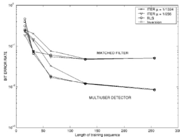
Figure 2. BER performance comparison of the iterative scheme with RLS and true inversion for different preamble lengths. This figure shows the error performance for two detectors, a MF detector and a multiuser detector.
