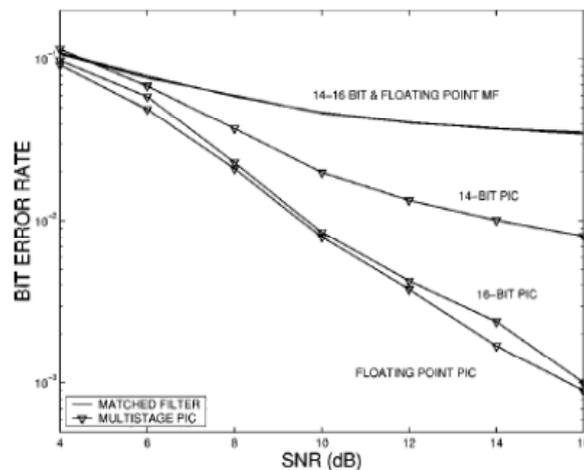
Figure 4. Fixed point error rate performance for  $N = 32$ ,  $K = 15$ . The figure shows the effects of quantization on the MF and MUD for different precisions.
