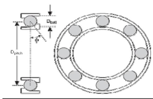
Figure 3. Roller Bearing geometry
