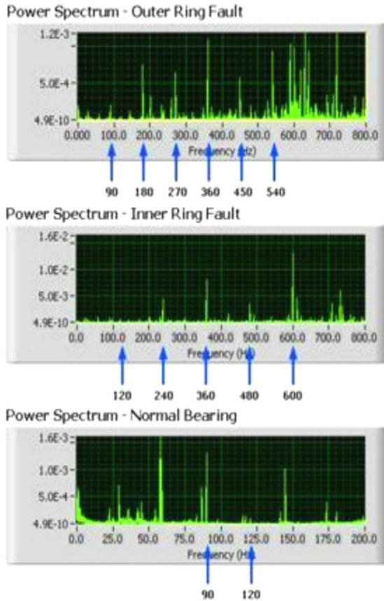
Figure 4. Illustration of vibration signature frequencies
