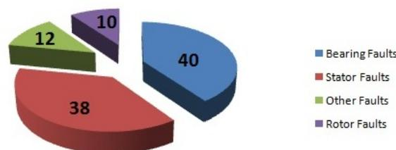
Figure 1. Fault Percentages in Induction Motor
