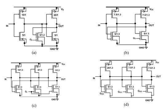
Figure 6. Electrical Scheme of Schmitt Trigger based on DCG-FGT.
