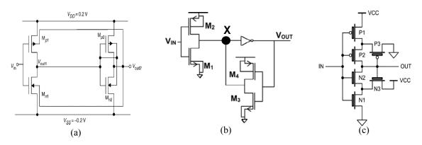
Figure 4. Traditional electric scheme of Schmitt trigger.
