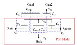
Figure 3. Electrical equivalent circuit of DCG-FGT transistor.
