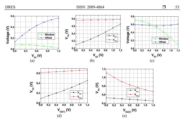
Figure 7. Simulations of the Schmitt triggers based on DCG-FGT transistor
