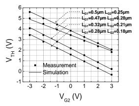
Figure 2. Measured and calculated threshold voltage values versus V<sub>G2</sub> for different length ratio configurations
