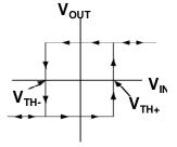
Figure 5. Characteristic of Traditional electric scheme of Schmitt trigger. 4. Adjustable Schmitt trigger based on DCG-FGT transistor
